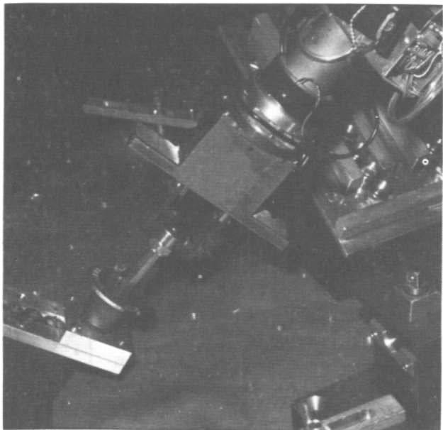
Figure 2. Sprinkler Assembly Fixture with Manipulator Hand and Force Sensing Wrist.
