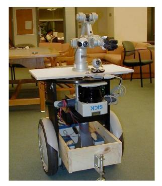
Fig. 7. The STAIR robot. The 5-dof arm was used to pick up the objects.
