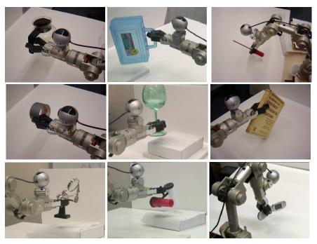
**Fig. 6.** The robotic arm picking up various objects: jug, box, screwdriver, duct-tape, wine glass, book, a chip-holder, powerhorn, and cellphone.
