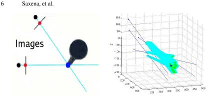
**Fig. 5.** Statistical Triangulation of the grasping point. (a) A sketch showing rays from two images intersecting at the grasping point (shown in dark blue). (b) A 3-d plot showing multiple Gaussian cones (in light blue) from 3 images, intersecting at the grasping point (shown in dark blue).
