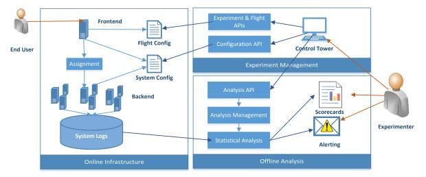
Figure 3: Experimentation System Architecture
