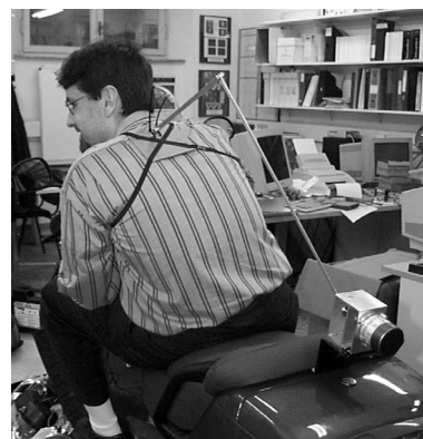
Figure 2. The encoder measuring the rider's lateral lean angle
