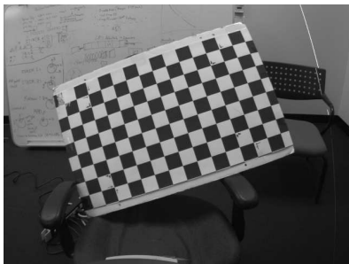
Fig. 5. An image of a (distorted) checkerboard and a laser beam captured by camera 2 (right corner).
