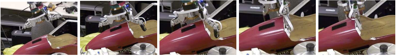
Fig. 7: A sequence showing the grasp trajectory chosen by our algorithm. Initially, the fingers are completely open; as more data comes, the estimates get better, and the hand turns and closes the finger in such a way that all the fingers touch the object at the same time.
