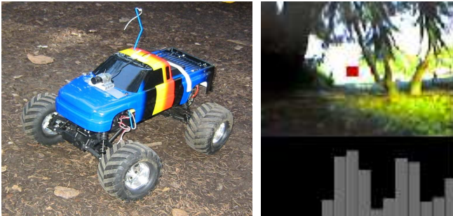
Figure 6: (Left) The remote-controlled car driven autonomously. (Right) A view from the car, with the chosen steering direction indicated by the red square; the estimated distances to obstacles in the different directions are shown by the bar graph below the image.
